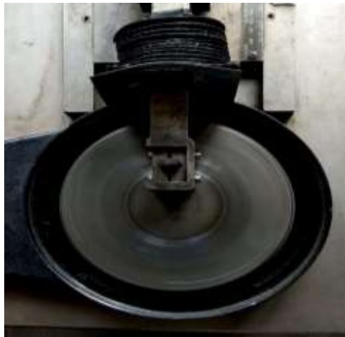
Figure 9 mounting of specimen on tribometer
