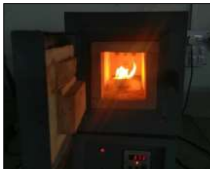
Figure 8 furnace used for flame resistance
